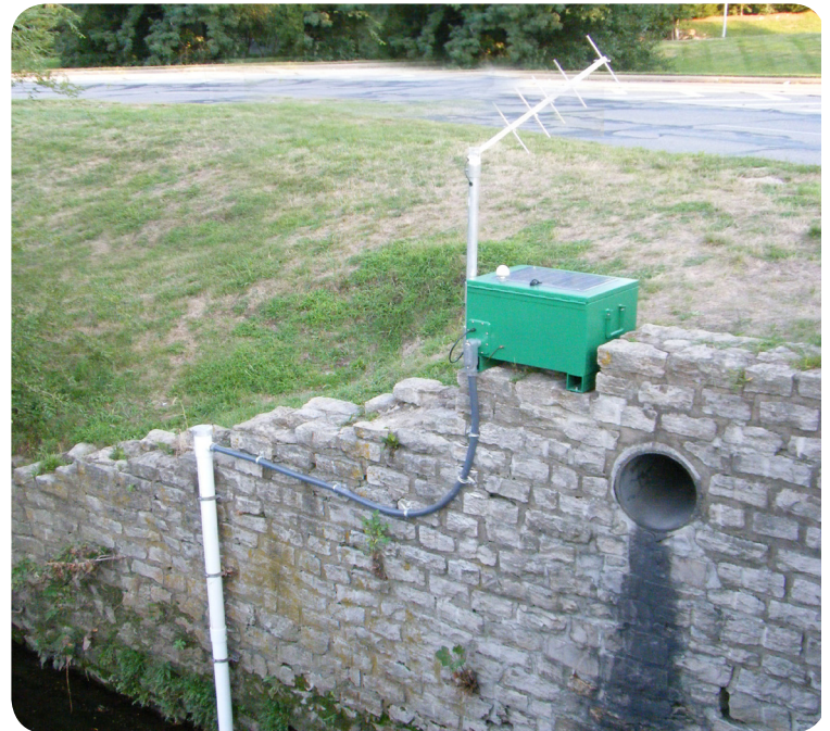
Portable aluminum chest monitoring system containing YSI Sonde and Data Logger. Kansas City, Kansas
