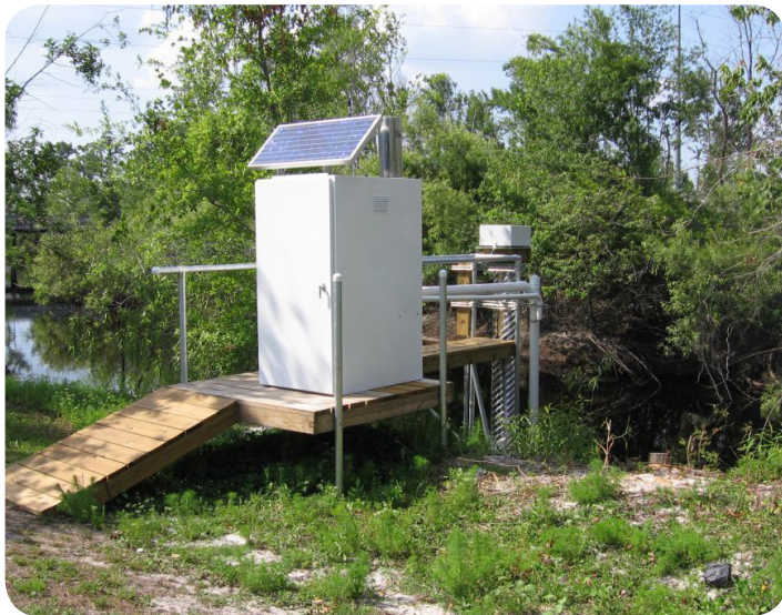
Stormwater monitoring site containing SonTek-SL, YSI Shaft Encoder, Level Sensor, Sonde, Portable Water Sampler, Rain Gauge, Data Logger, and Solar Panel. Kissimmee, Florida
