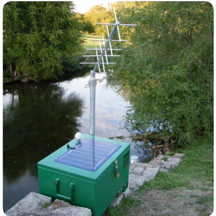
Portable aluminum chest monitoring system containing YSI Sonde and Data Logger. Kansas City, Kansas
